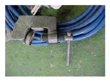
(h) Apply the earth end clamp by hand and tighten, using only the tommy bar on the clamp, and check that it is secure.
