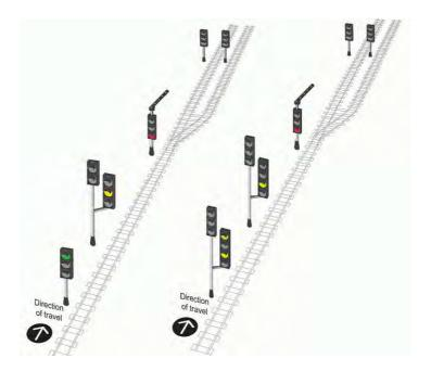
Splitting distant signals with junction signal at danger where there is a right-hand diverging route
