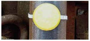
**Detonator secured to rail**
