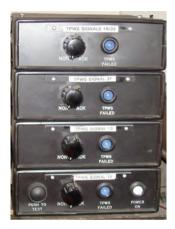
Example of a failure indication unit
