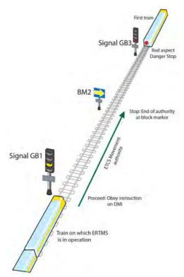
A train on which ERTMS is operating can be issued with a movement authority (MA) to any intermediate block marker. In this case signal GB1 will display a yellow aspect.
