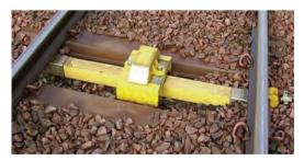
An example of a portable magnet
