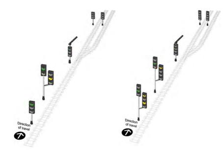
Splitting distant signals with junction signal cleared for the straight route where there is a right-hand diverging route
