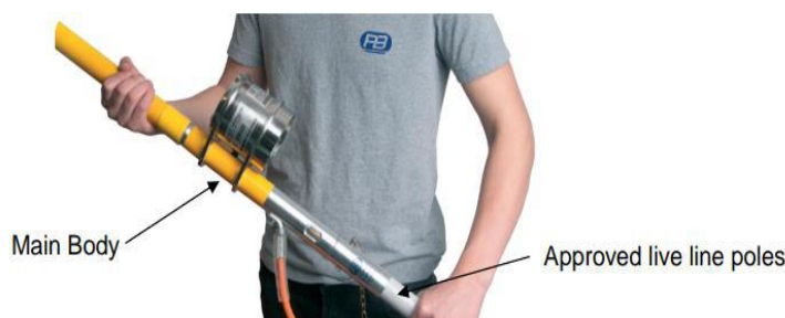
Figure 4 – Attaching the assembled C31 LLI to approved live line poles
