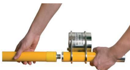
Figure 2 – Screw the high voltage probe to the main body
