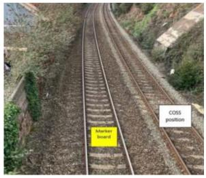
Permission to place the marker boards had not been given by the ES and both lines were still open to traffic. The forward-facing CCTV footage from the train shows the COSS moving clear from the down line 4 foot into the open Up line with less than 3 seconds to spare before the train hit the markerboard.
